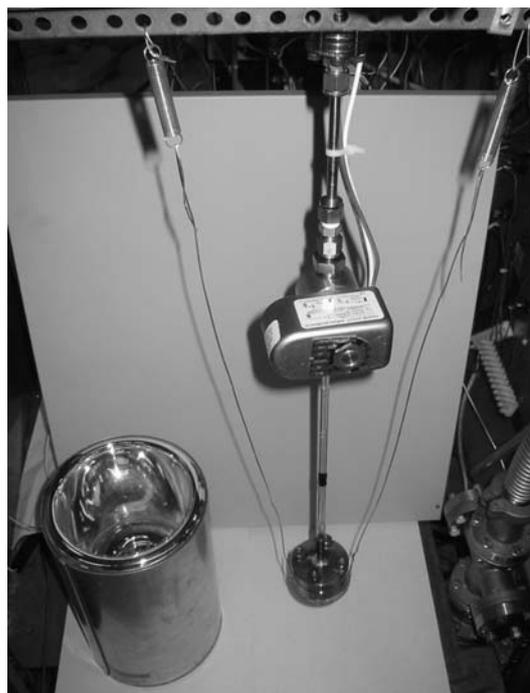
**Fig. 2** Complete adsorption cell attached to system valve and supported by springs. The entire cell is immersed in the Dewar (left) until the level of the cryogenic bath is up to the bottom of the black tape
